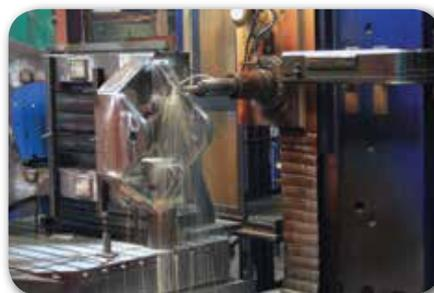
*Machine working is carried out in larger CNC operated mill boring machines.*
