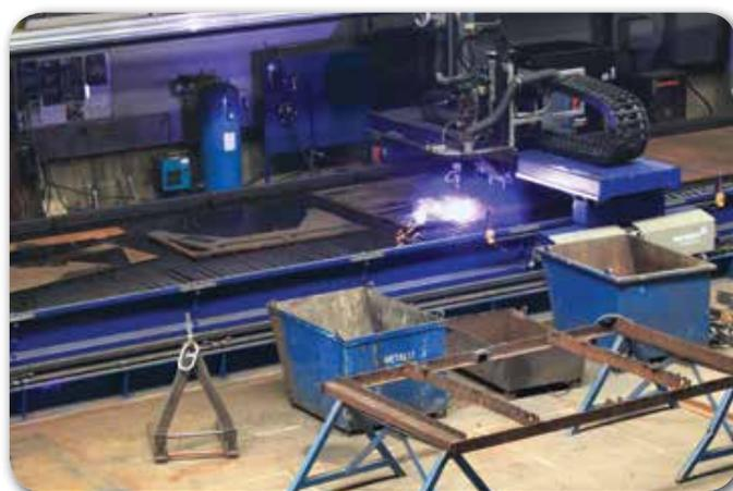
*Cutting is done with plasma cutting (with bevel cutting) and oxygen cutting.*
