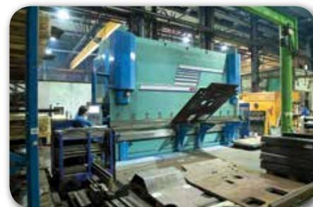
*Bending takes place in 630-ton press brake with a length of 6 m.*
