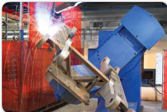
Welding is performed manually and with robot welding
