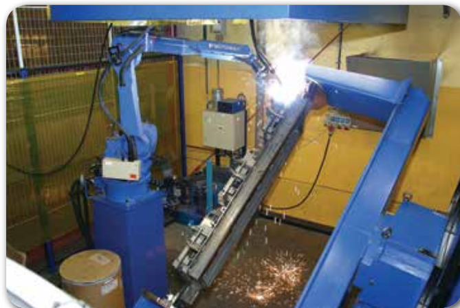
Welding is performed manually and using robotic welding
