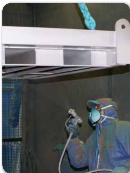
Spraying done in a painting chamber with heat recovery and two drying ovens. We can paint up to level C5-M
